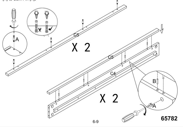
STEP 3: Insert the dowels(B) into the Top Bottom Panel (C2).Use a Hex Key (J) to assembe the Side Rail (C4) to the Headboard Bottom Panel (C2) with Bolt (A).Insert the Dowel (B) to the Footboard (C3).Use a Wrench (L) to assembel the Side Rail (C4) to the Footboard (C3) with Bolt (C). then Insert the Cover (M) to the Side Rail (C4).
